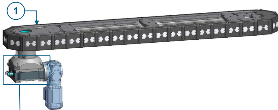
Fig. 5 Nameplate (1) Nameplate position LFA
